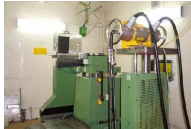
Fig. 2 Scanning system showing mechanical manipulator, X-ray tube-head and detector
